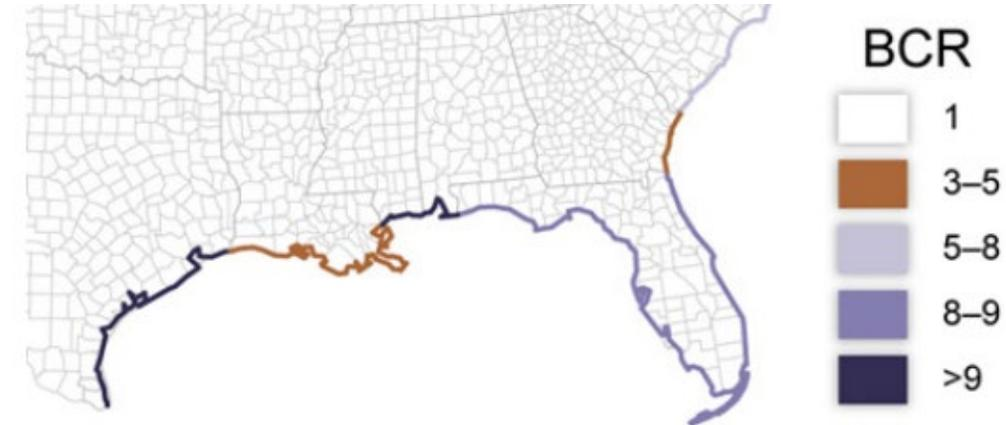
**FIGURE 2.** BCR of coastal flooding mitigation by elevating homes above 2015 IRC requirements (by state).
